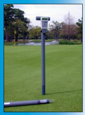
The TH<sub>2</sub>O takes accurate soil moisture samples with minimal disturbance. By simply inserting the probe into the ground, actual soil moisture percentage readings are given. Watering needs can be quickly determined making it easy to remove the guesswork and errors.
