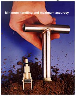
The En Core® Sampler is made of high-tech inert composite polymer and is available in 5 gram and 25 gram versions.
