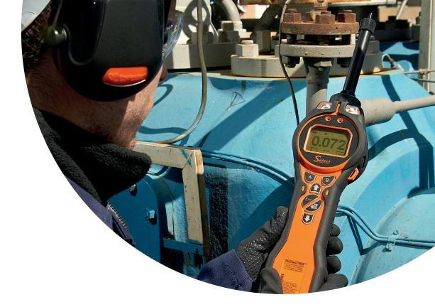
A revolutionary hand-held detector, Tiger Select can be operated either with a benzene pre-filter tube to detect benzene selectively, or without to detect total aromatic compounds (TAC). For simplicity and ease of use, the Tiger Select has been split into two, user-friendly modes: Basic and Advanced. Both modes are user-selectable.
