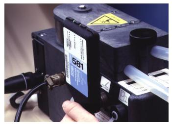
The Isco 581 RTD provides a fast, simple way to collect and transport data from 6700 Series Samplers.
