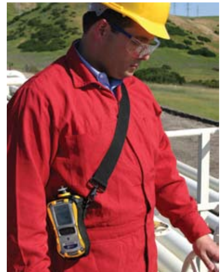
MultiRAE used for worker exposure monitoring at an oil refinery
