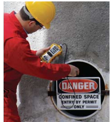
Confined space testing with the MultiRAE Lite
