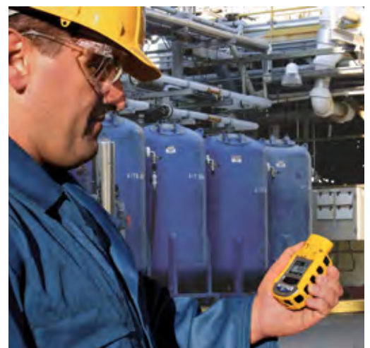
Worker exposure monitoring with ToxiRAE Pro PID at a PVC plant
