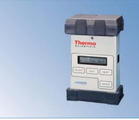
The Thermo Scientific personal DataRAM pDR-1000AN Monitor is a passive sampling, light-scattering nephelometer that measures real-time mass concentrations of dust, smoke, mists, and fumes in industrial as well as other indoor and outdoor environments.
