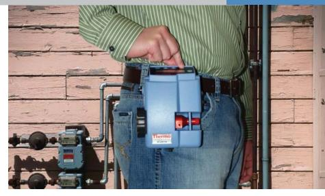
The Thermo Scientific personal DataRAM, pDR-1500 was developed to meet a need for a fully integrated, active sampling personal scale instrument with greater accuracy, increased capabilities, low size and weight, maximum ease-of-use and increased operating time.
