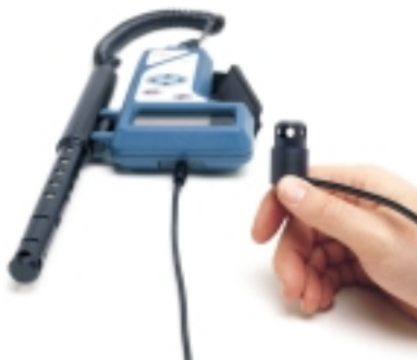
Auxiliary port permits use of an optional, secondary temperature sensor.
