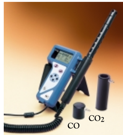
Calibration collars make recalibrating simple and quick in the field.
