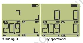
Once all sensors have completed the warm up sequence the detector is ready to detect all gases.
