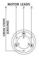
**NOTE:** For Tefzel motor lead, use the following wiring pattern: 1, 2, 3 clock wise from ground terminal (striped green).
