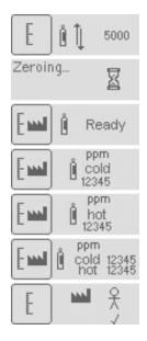
\* Fill an empty (uncontaminated) sample bag with 5000 ppm Helium gas before starting the calibration procedure. Also remove the outer grey probe from the GasCheck Tesla.
