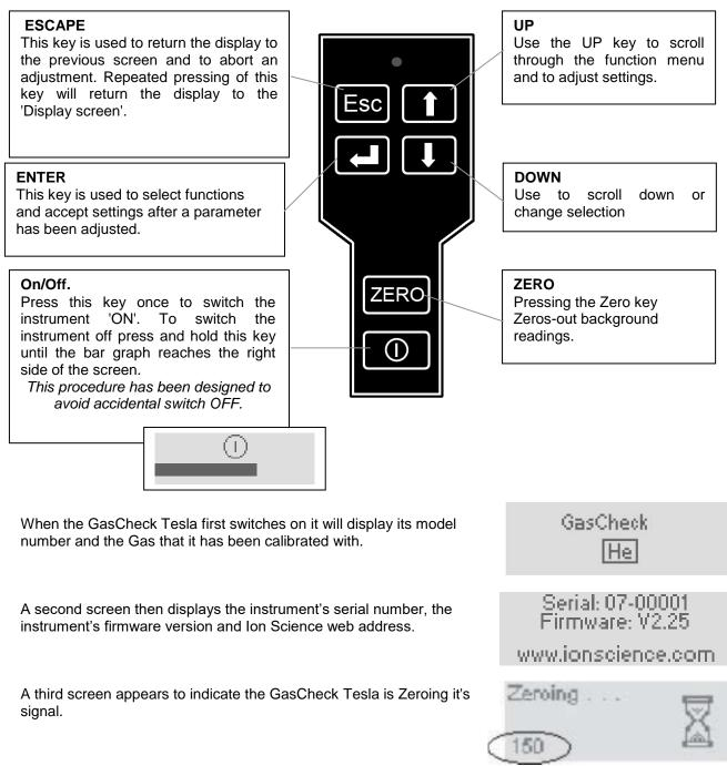
Once the Zero routine is complete the instrument displays it's running screen and is ready for use.
