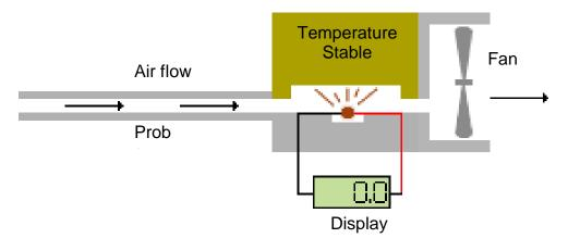
When gases with different thermal qualities pass through the chamber the amount of heat being transmitted to the Temperature Stable block changes. These changes are measured, calculated and displayed on GasCheck Tesla as leak rates or gas concentrations.
