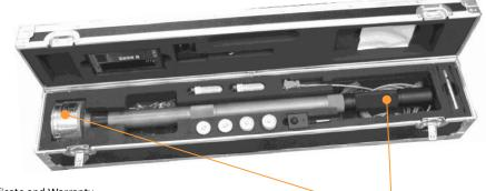
The GasClam 2 is packed for transport with caps on the inlet, outlet and vent barbs, these <u>black caps</u> must be removed before the Unit is used. If it is intended to store the Unit for a longer period of time it is recommended to replace the caps on the barbs to stop moisture and dust ingression.
