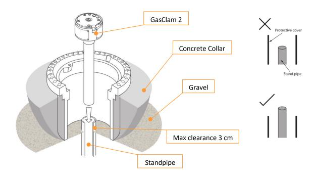
It is important to have the standpipe a maximum of 3 cm above the base of the Headworks, this will ensure the GasClam 2 will fit under the lid of the cover. The Headworks must be concentric to the standpipe for the GasClam 2 to be housed correctly. The standpipe must also be cut square to allow a good seal.
