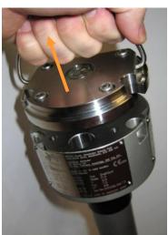
If this procedure is not followed carefully, damage to the O-ring may be caused compromising the intrinsic safety of the Unit.
