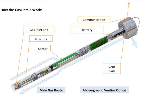
When logging is started the GasClam 2 instantly takes its first sample. A click is heard and then the pump starts which takes a sample of air from the borehole. First the pressure and temperature readings are taken. While the pump is on readings from gas flow sensors are taken. The pump then switches off and after a short pause readings from static gas sensors are taken. The whole process takes approximately 2 ½ minutes depending on sensor configuration.
