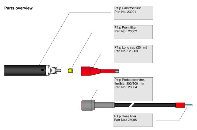
The **ISM** front filter optimises the replacement process for the suction filter as well as the service life of the SmartSensor, which essentially depends on the amount contamination from the ambient air flowing into the ionisation chamber.
