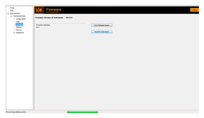
When you are ready to send the new Firmware to the instrument. Select 'Send to Instrument'.
