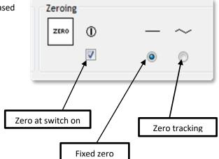
The zero functions may be enabled or disabled by ticking or un-ticking the box. Constant or tracked zero is selected by use of the radio buttons associated with the icons.
