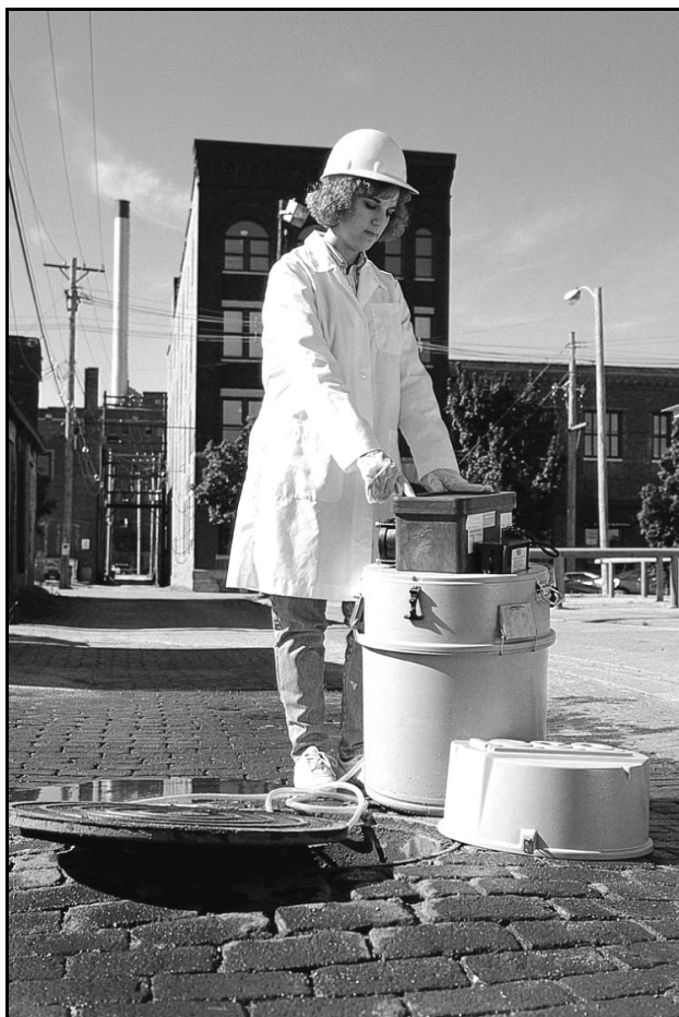
Figure 6 Placement of the Sampler Adjacent to Manhole
