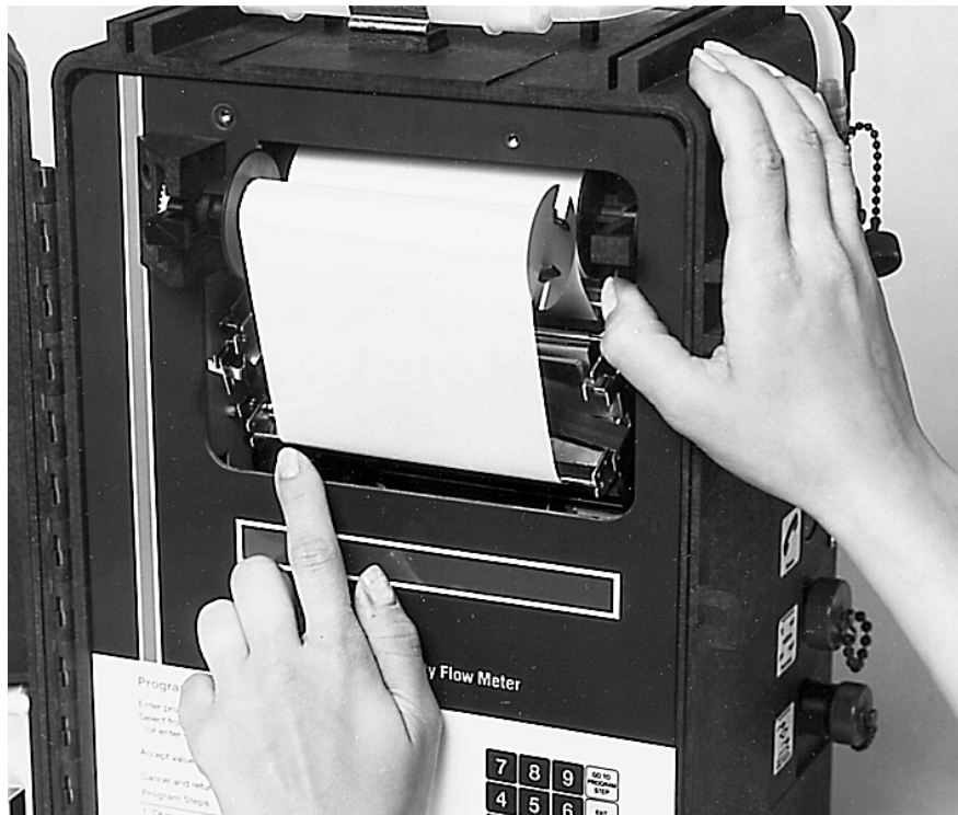
Figure 5-4 Lifting the Flow Meter from the Case
