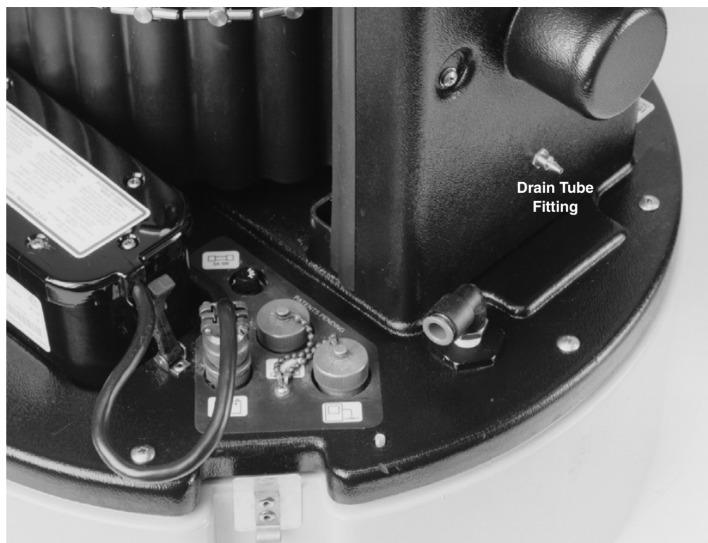
Figure 1-6 Power Source, Connectors, and Drain Tube Fitting
