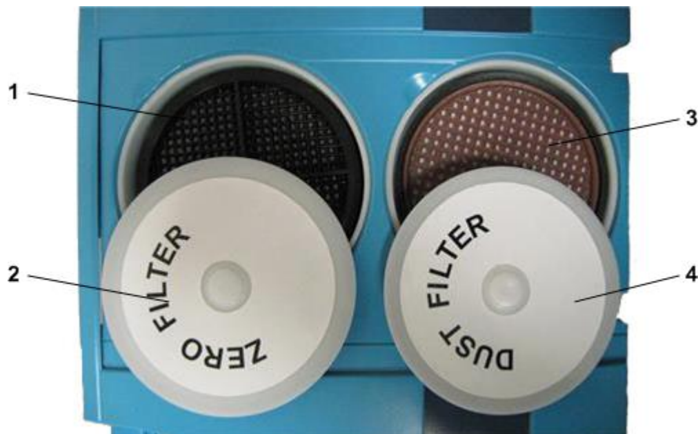
Fig. 3-1 - Location of the sorption and dust filters of RA-915M analyzer
