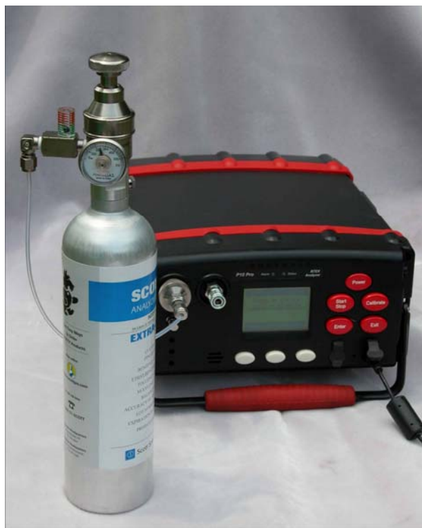
Figure 8. Calibration with Flow Match Regulator
