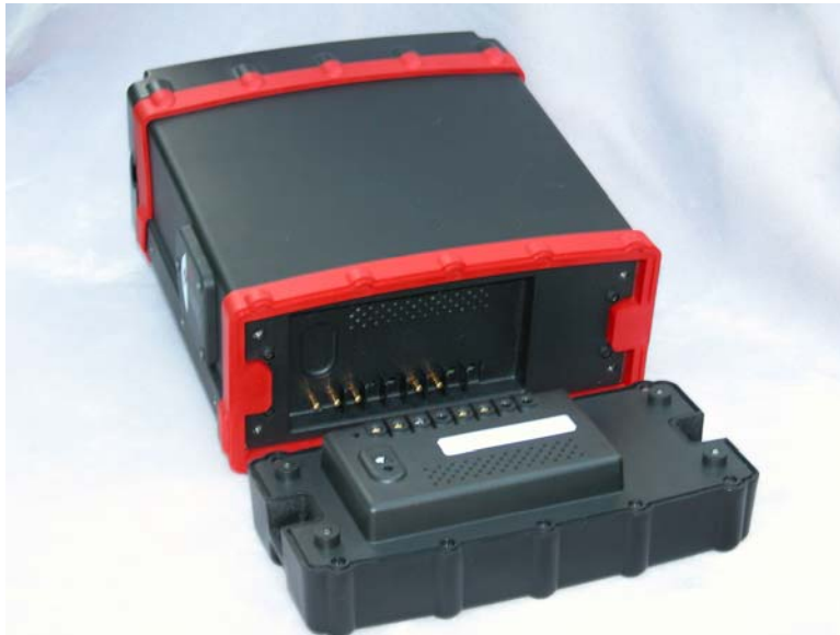
Figure 26. Battery Pack Removed
