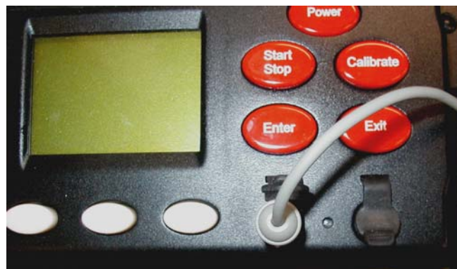
Figure 11. Connecting the Download Cable to the PetroPRO
