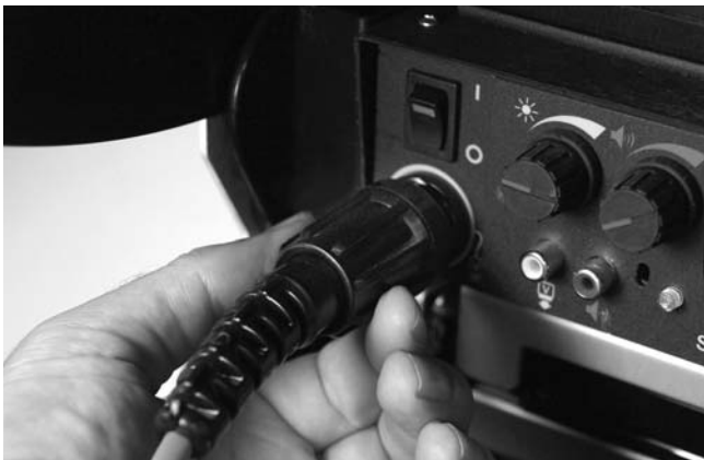
Figure 24 – Connecting System Plug To CCU
