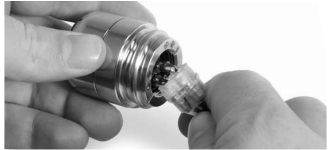
Figure 38 – Unplugging The Camera Head
