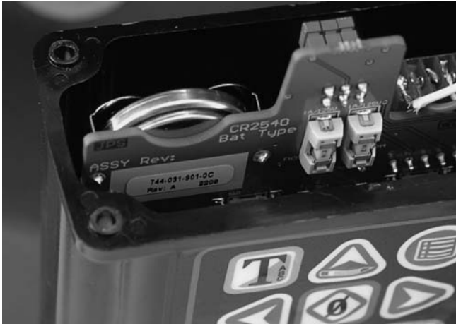
Figura 40 – Pila del CountPlus
