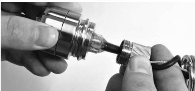
Figure 37 – Separating Locking Sleeve From Camera Head
