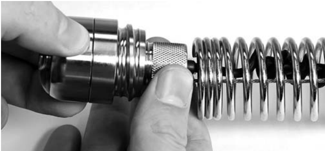
Figure 36 – Removing Camera Head From Locking Sleeve
