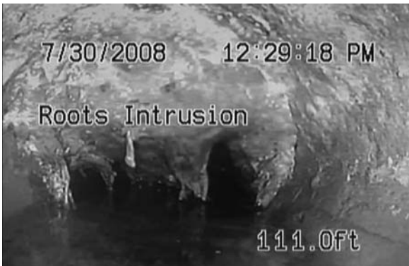
Figure 30 – Display Screen With Slide Text, Time and Distance Shown (Distance Measured From System Zero-Point)
