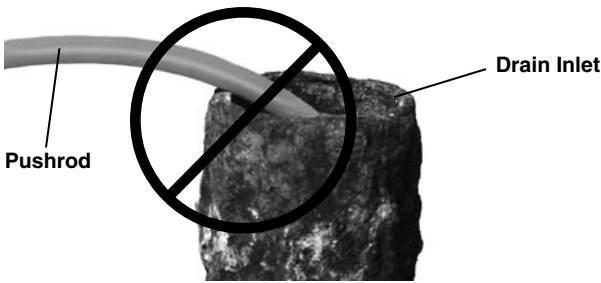
Figure 33 – Avoid Pulling At Sharp Angles
