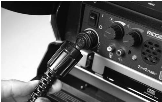
Figure 23 – Aligning System Cable Plug
