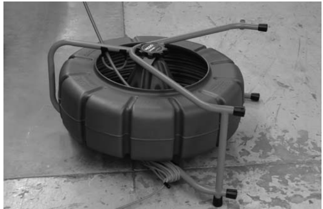
Figure 22 – Reel Can Be Positioned On Its Back For Greater Stability
