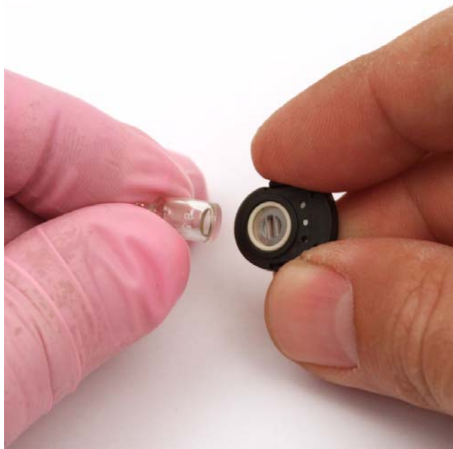
Figure 32: Reinstalling the Electrode Lamp
