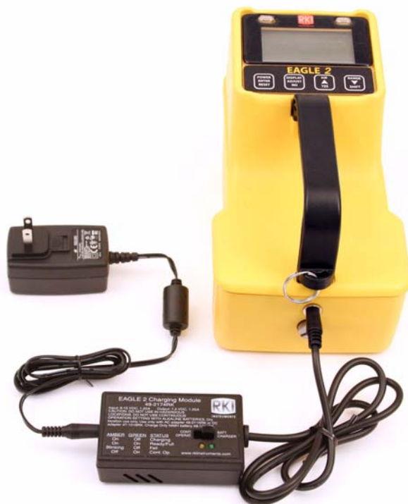
Figure 18: Connecting the EAGLE 2 to the Charger
