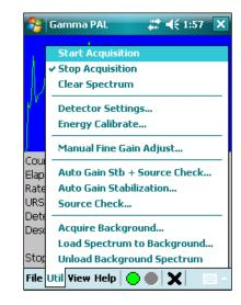
c. **Util**|**Clear Spectrum** performs an identical function to the black X on the button bar; it will clear the spectrum (after giving a warning and an opportunity to cancel the deletion).
