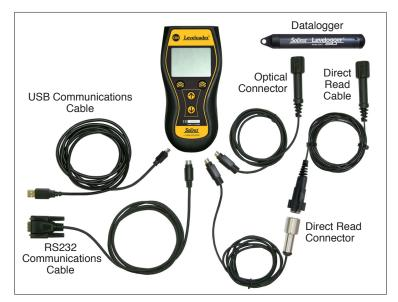
Figure 6-2 Leveloader Gold Connections
