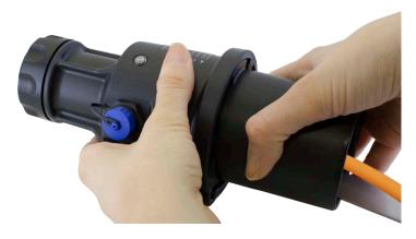
Slide the well cap sleeve up to the Wellhead and twist the well cap sleeve into the Wellhead until it seats.
