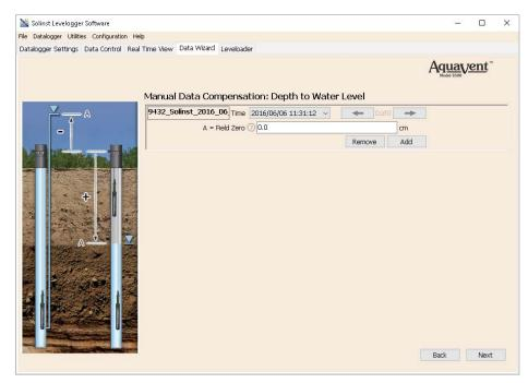
Figure 6-5 Manual Data Adjustment - Depth to Water Level
