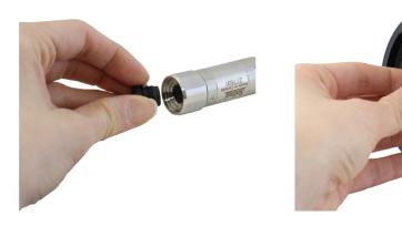
Remove the storage caps from the connectors on the Wellhead and Vented Cable.
