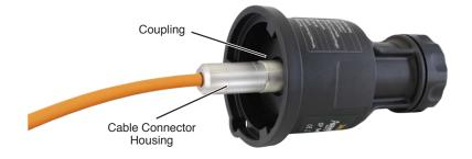
Twist the stainless steel coupling while holding the stainless steel cable connector housing still. Twist the stainless steel coupling until it seats. **Do not twist the Vented Cable or Wellhead.**
