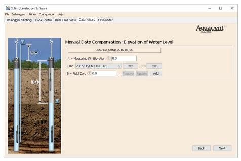
Figure 6-6 Manual Data Adjustment - Elevation of Water
