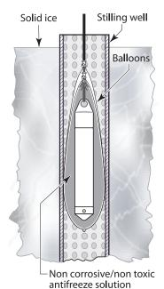
Figure 10-15 Installation in Freezing Liquid
