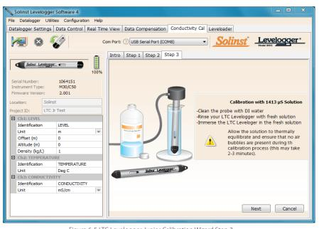
Figure 6-5 LTC Levelogger Junior Calibration Wizard Step 3 (example of window calibrating with 1413  $\mu$ S/cm solution)
