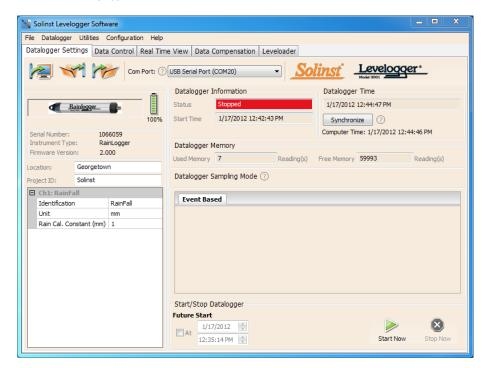
Figure 5-4 Rainlogger Channel Setup - Firmware 2.000 and up
