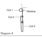
Figure 10-3 Wireline Hook Installation
