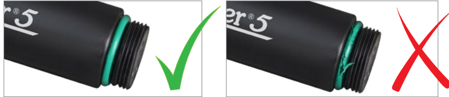
Figure 10-25 Levellogger O-ring Damage
