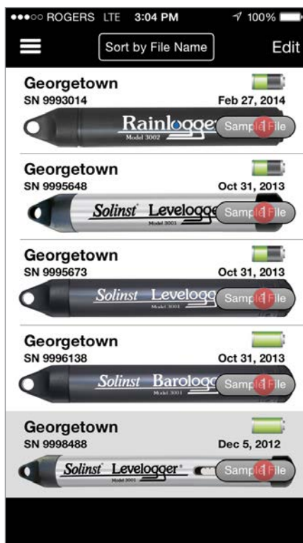
Figure 4-1 Solinst Levelogger App Home Screen on iOS - No Datalogger Connected
