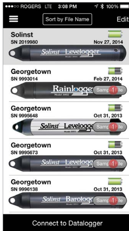
Figure 4-9 Connecting a Datalogger from the Dataloggers Screen - iOS
