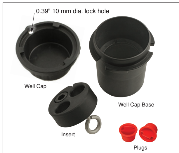
Figure 10-8 Model 3001 Well Cap Assembly (#110099)
