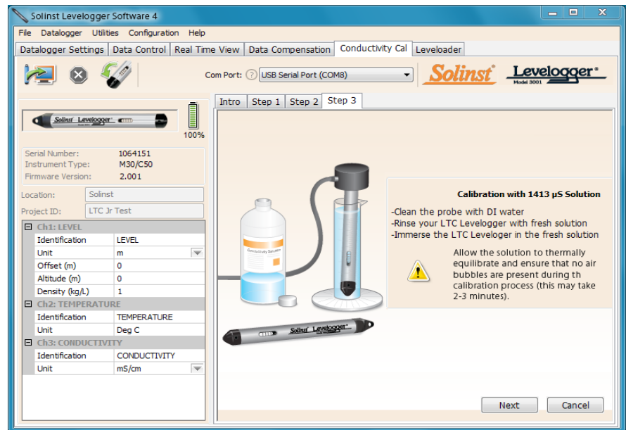
Figure 6-5 LTC Levellogger Junior Calibration Wizard Step 3 (example of window calibrating with 1413 µS/cm solution)
