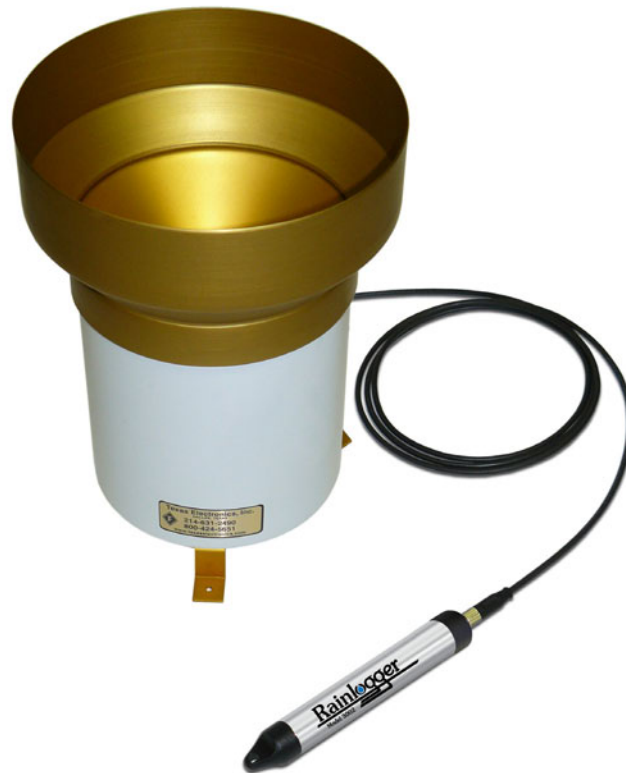
Figure 10-14 Rainlogger Connected to Tipping Bucket
