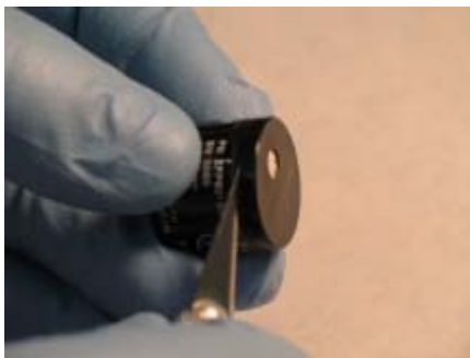
Figure 7-4. Removing the Filter Cap
