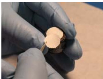
Figure 7-14. Placing the Filter Media
