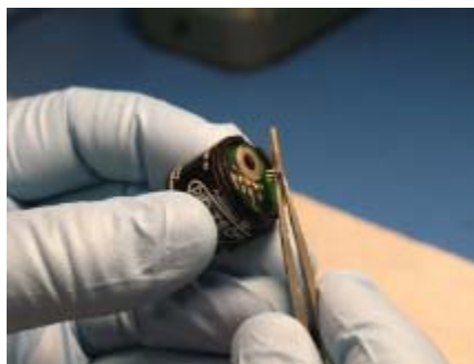
Figure 7–12. Installing the Cell Assembly
