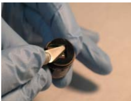
Figure 7-6. Removing the Spacer
