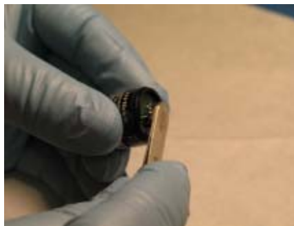
Figure 7–11. Pressing Down the PID Lamp
