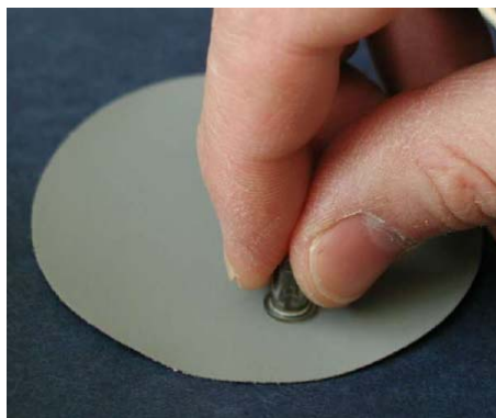
Figure 7-9. Cleaning the PID Lamp
