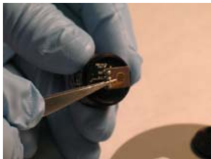
Figure 7-7. Removing the Cell Assembly
