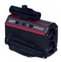
**LaserTech** Rangefinder: This is also a good choice for distance and vertical angles, but it does not have Bluetooth, so the GPS cannot interface with it, so you need to record data, either in a notebook or entering offset values using the Options button in the Terrasync Data collection screen. Use a handheld **compass** or the Mapstar compass module (you may want to let Terrasync do the magnetic declination correction).
