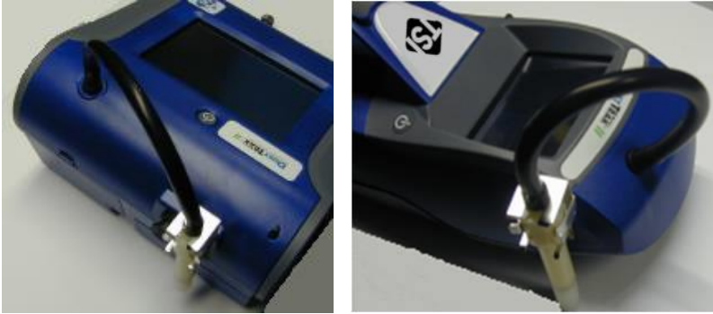
Figure 2-8: Installing Door-Oliver Cyclone
