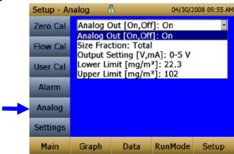
**Analog** setup screen sets the parameters that will drive the analog out port. Applies to the 8533 Desktop model only.
