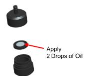
Figure 4-4: Apply 2 Drops of Oil to Impactor Plate
