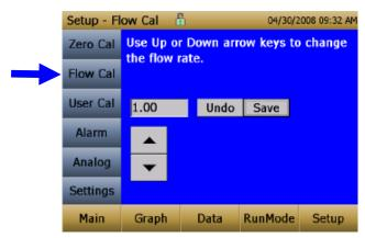
6. Conduct a preflow calibration on the DustTrak monitor using the same kind of sample media you will sample with. Now, attach the sample media you intend to sample with and start sampling aerosol for the desired time. After the desired run time, stop the sampling. Remove the
