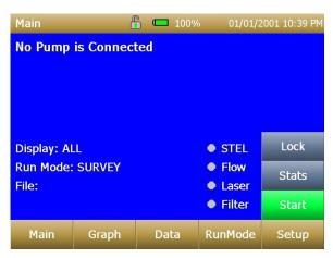
Connect the External Pump Module to the DustTrak monitor and then try again. TSI recommends powering down the DustTrak monitor before connecting the External Pump Module to the DustTrak monitor. Connect the power cable and the flow tubing between the DustTrak monitor and the External pump module, as applicable.
