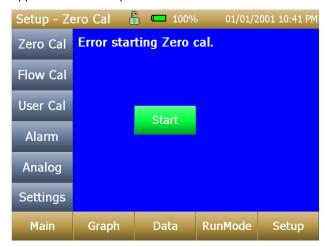
4. If the pump is **not** connected while attempting to perform a Flow Cal, an error appears on the Setup screen.
