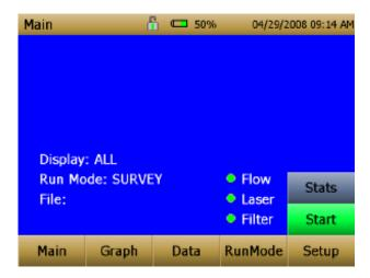
Using a stylus or fingertip, touch the "buttons" on the screen to activate different menus.
