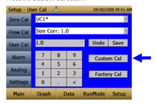
Follow the on screen steps to determine the size Corr. The PM<sub>2.5</sub> impactor is required for this step.
