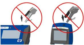
Figure 4-3: DO NOT Blow into Instrument
