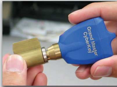
Figure 1-4: Configuring a CyberLock Using the Grand Master
