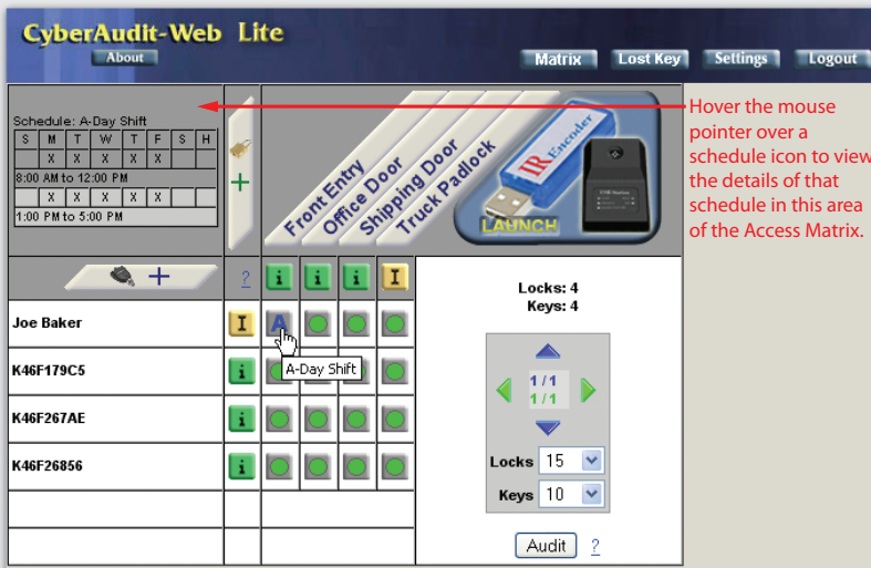
Figure 2-19: The Access Matrix Showing Schedule Details
