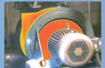
IR/Color Alarm Displays only temperatures falling above, below, or in between a user-selected range in infrared, and anything outside the selected range as a visual (visible light) image.
