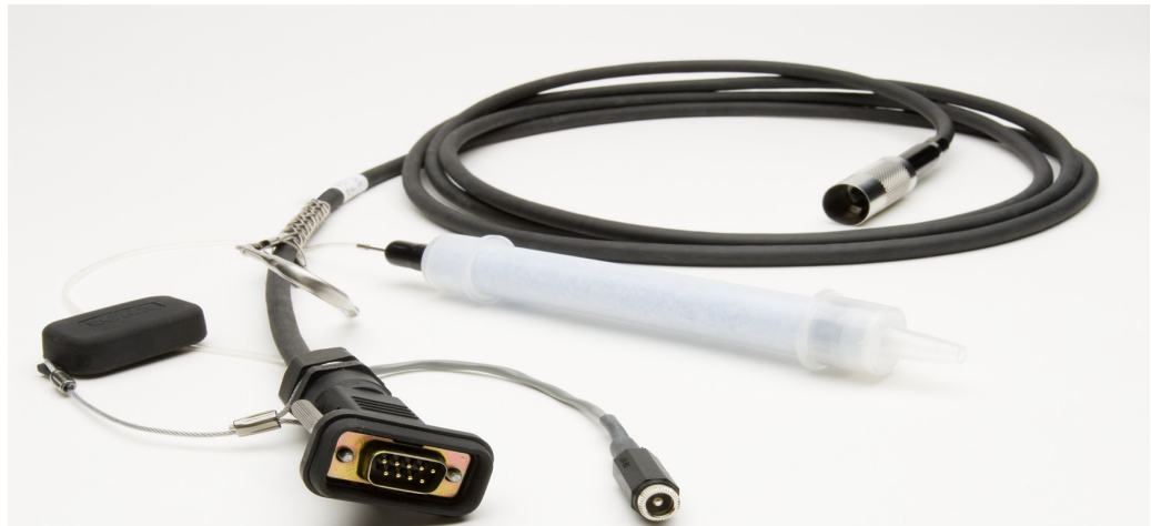
Model 710 (stainless steel) or Model 730 (titanium) Universal Cable assembly for atmospheric compensation for vented Level Scouts and direct data readout and communication to absolute or vented sensors while deployed in the field. Includes RS-485 connector, DC power connector, battery connector, and desiccant cartridge.
